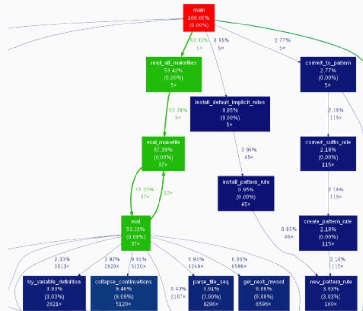
Perf is performance monitoring and analysis tool for Linux. It uses statistical profiling, where it polls the program and sees what function is working
